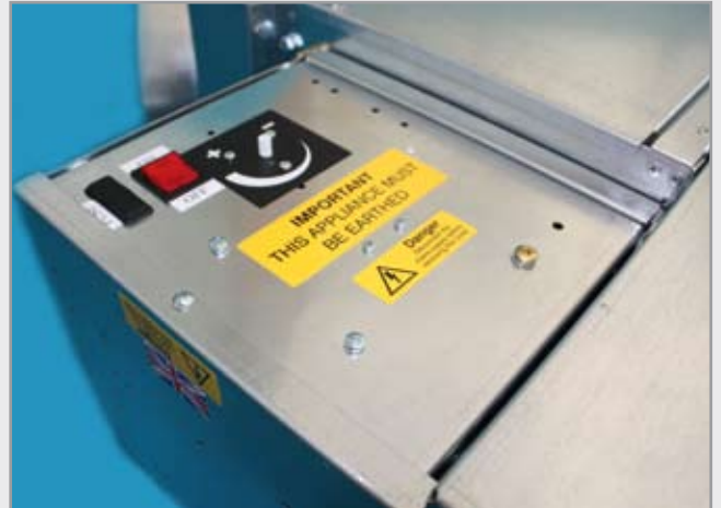
'Panther' control box with fitted speed potentiometer
