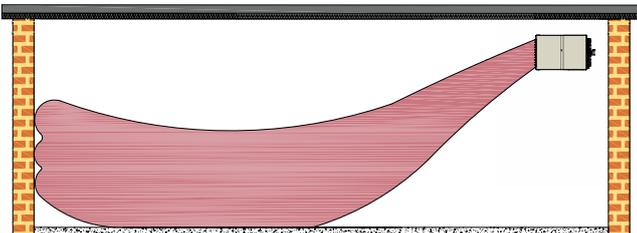
Longer air throws provide even heat distribution and reduce pre-heat times
