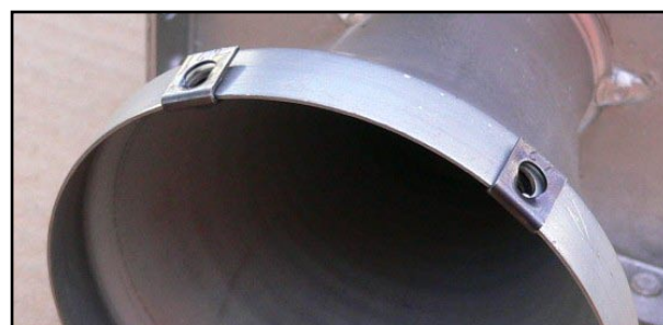
Fig. 15: Push speed nuts on venturi inlet
