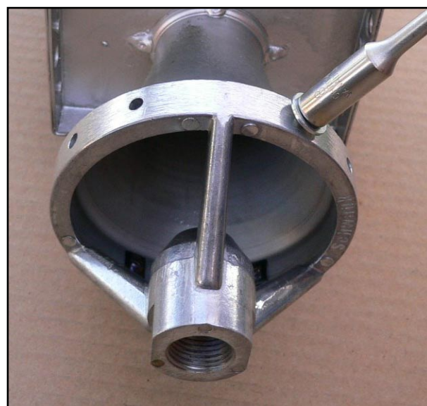
Fig. 16: Fix nozzle holder on venturi inlet
